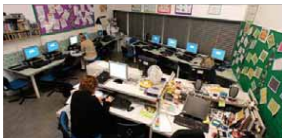
◀ Left Blinds are down in the ICT room, to prevent glare, but this forces the use of electric lights.
